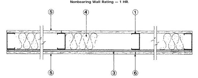
1. Studs — Channel-shaped, min 2-1/2 in. wide by 1-1/4 in. deep with 5/16 in. folded back return flange legs. Fabricated from No. 25 MSG galv steel. Max stud spacing 24 in. OC. Studs to be cut 1 in. less than assembly height.
